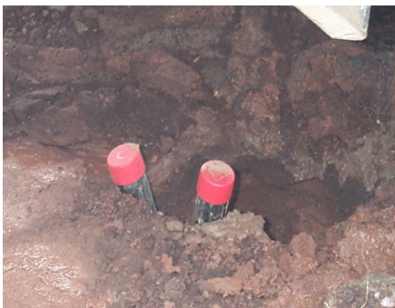
The borehole top showing the pipe
